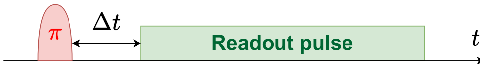
Figure 3.9: Pulse sequence diagram of a T_1 measurement. The qubit is excited with a \pi -pulse and let to decay during a variable time \Delta t before dispersive readout.
